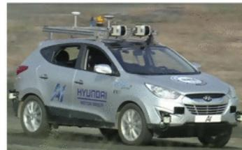
Figure 1. Autonomous vehicle A1.
